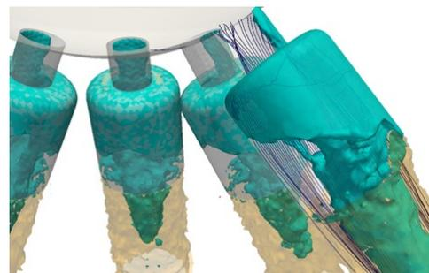
Simulation of flash boiling through stepped holes. The green surfaces show high concentrations of vapor.
